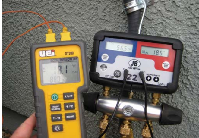
Fig. 5.21 Semi-automatic superheat and subcooling calculations Modern digital refrigerant gauges calculate subcooling and superheat semi-automatically, based on temperature and pressure measurements and their built-in refrigerant property tables. This saves time and improves both accuracy and consistency of these critical measurements.
