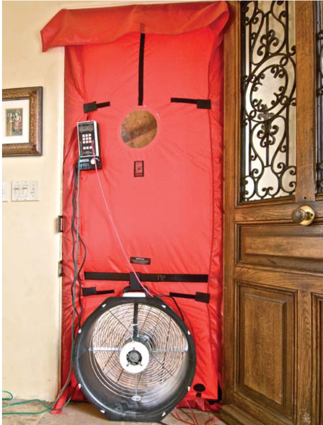
Fig. 3.8 Blower door for in-process measurements as the workers are sealing the attic and crawl space
