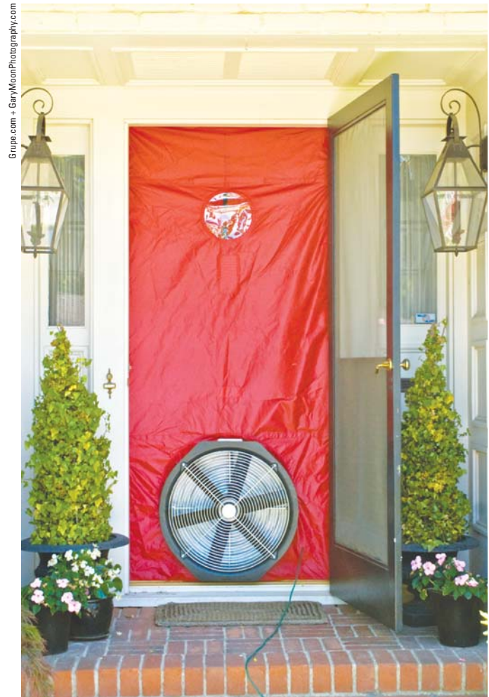
Fig. 9.3 Blower door testing is repeated periodically during air sealing operations to provide feedback to the crew about their progress towards their air tightness target.
