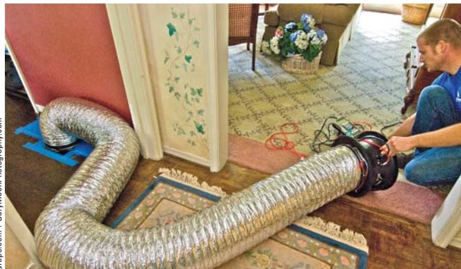
Fig. 5.19 Duct blaster, used in combination with the blower door for measuring duct leakage to the outdoors
