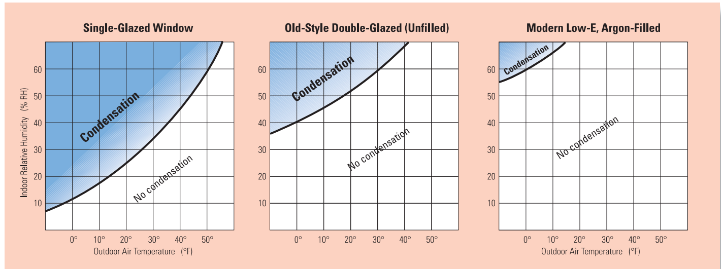
Fig. 10.6 Condensation risk of glazing alternatives
