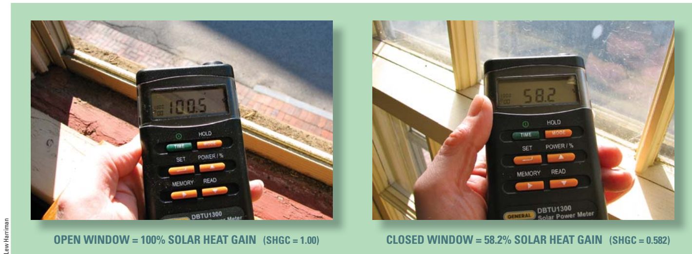
Fig. 5.25 Solar power meter measures solar heat gain coefficient (SHGC)
