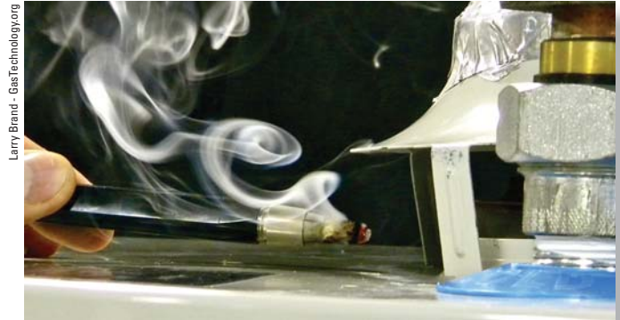
Figure 5.8 Tests are important to avoid backdrafting and spillage from natural draft appliances after the house is tightened up
