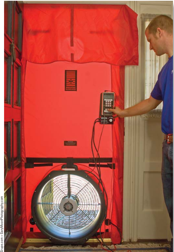
Fig. 2.4 In-process measurements provide essential feedback If there's a secret to the success of Home Performance Contracting, it's the instant feedback to installation crews provided by in-process measurements of successful installation.
