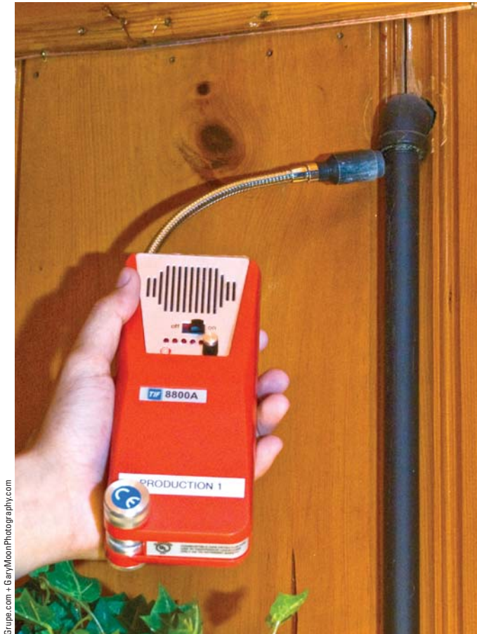
Fig. 5.13 Electronic gas leak detector - Audible indicator
