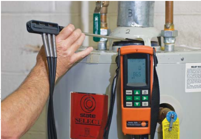
Fig. 5.12 Carbon monoxide probe location Note how the probe is inserted slightly downwards into the exhaust stack. In that location, there's not yet any ambient air diluting the gas and distorting the reading, as would be the case just an inch higher up in the stack.
